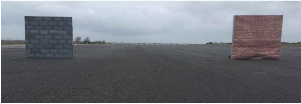
Image shows both MD-Wall and Real wall. The real wall was the exact location of the test, MD-Wall moved to this location.
